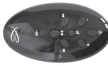
Activate a playback component, for instance turn the TV set on: Stream 3 automatically turns on, the POWER LED turns from red to green and flickers during the 40 seconds initialisation period, then remains on.
